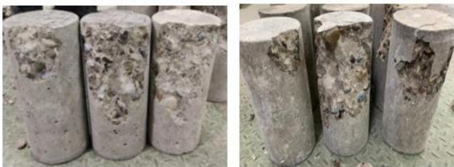
Figure 5. Typical cylinder failures tested at 7 and 28 days.
