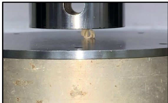
Figure 4: Universal Testing Machine with composite sample fracture
