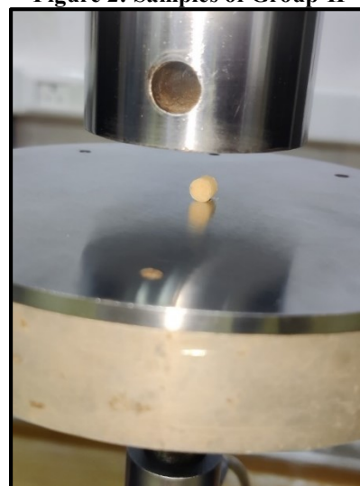
Figure 3: Universal Testing Machine with Composite Sample
