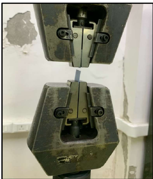
Figure 3: Digital Universal Testing Machine (UTM) with alginate sample failure
