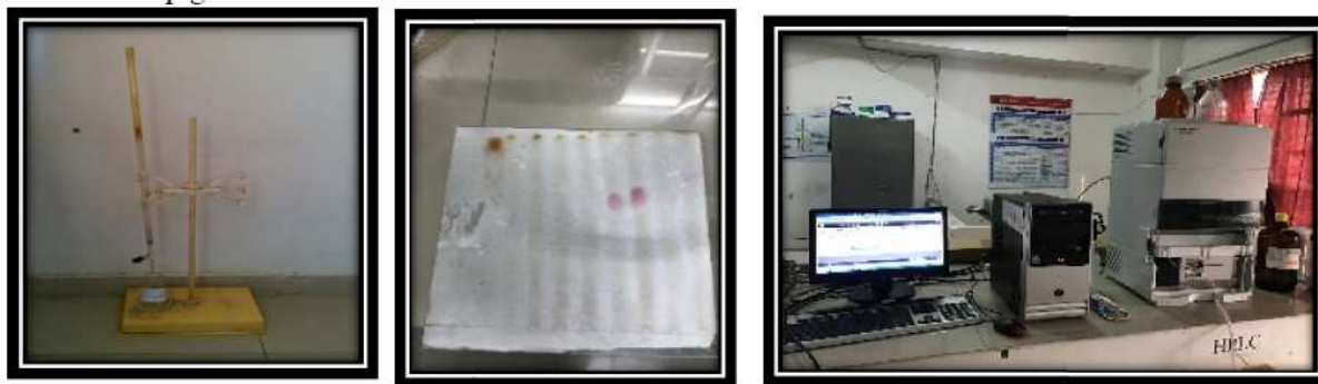
Figure 6: (a) Glass column used as column chromatography for the purification of Allium sativum (b) Thin Layer Chromatography of Allium sativum (c) High Pressure Liquid Chromatography of Allium sativum extract
