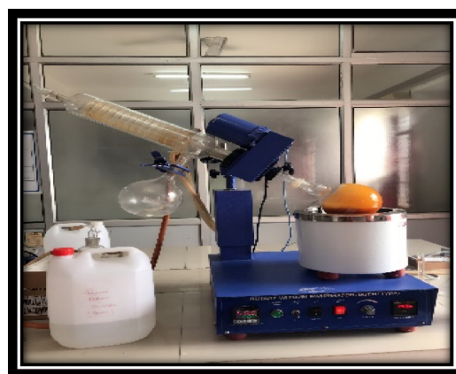
Figure 4: Rota evaporator concentrating Allium sativum extract
