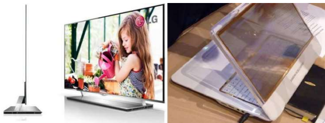
Figure 8: a: Full-HD AMOLED TV (4mm thick and weighs just 3.5 Kg); b: Transparent OLED Laptop.
