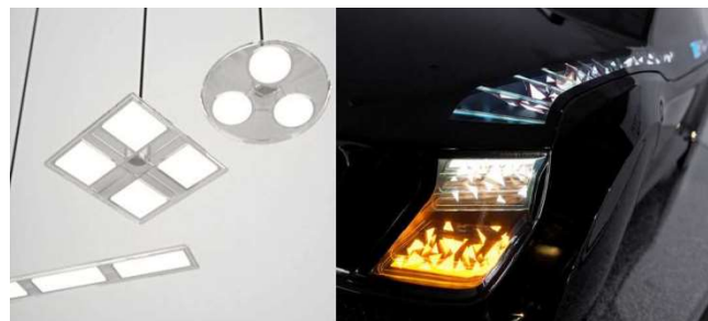
Figure 10: a: White OLED flat Lamps; b: White and other colors OLED used in car lighting
