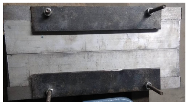
Figure 2: Clamping of Al strip on cast iron bed
