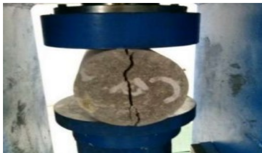
Figure 1.6 Split Tensile test on Concrete
