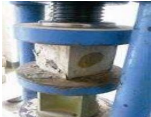
Figure 1.5 Compression test on Concrete Cube
