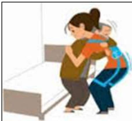
The advanced technology utilized for designing robots that protect our back with the power application of rubber! “Smart Suit Lite” is a hip supporter that alleviates fatigue by utilizing the tension of rubber bands. It prevents strain on the back by helping the movement of lifting the upper part of the body from a semi-crouching position, and by tightening the body trunk [7].
