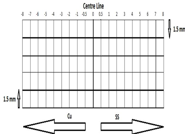
Fig.2: Orientation of microhardness measurement.
