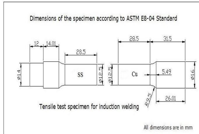
Fig.3: Dimension of Tensile specimen according to the ASTM E8-04 Standard.
