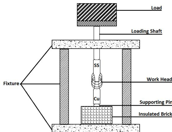
Fig.1: Induction welding setup.
