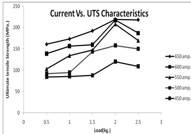
Fig.8: The behavior of UTS of induction welded specimen Cu and SS(AISI304L) for different current settings and loads.
