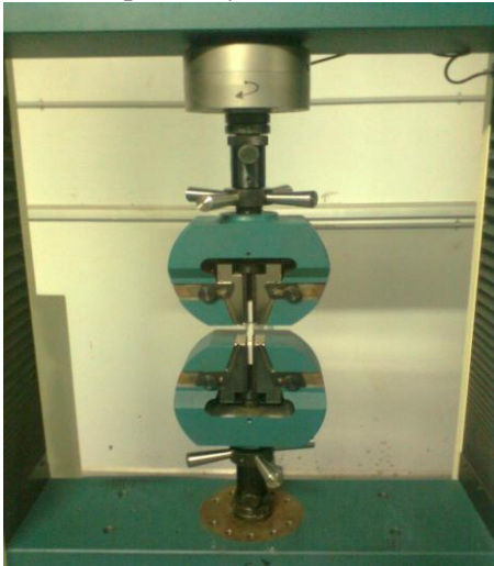
Fig.2 Tinioulesen universal testing machine
