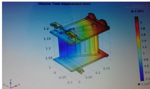
Fig.No.4. Surface plot of the displacement
