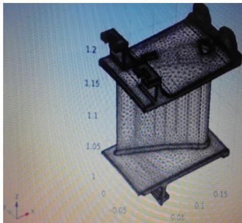
Fig.No.2.Creating Mesh Turbine Stator Blade.
